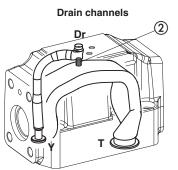
Internal piloting: Without blinded plug SP-X300F ①; External piloting: Add blinded plug SP-X300F ①; Without blinded plug SP-X300F 2; Internal drain: Add blinded plug SP-X300F ②. External drain:
