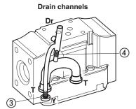
Internal piloting: blinded plug SP-X300F ① in X;
