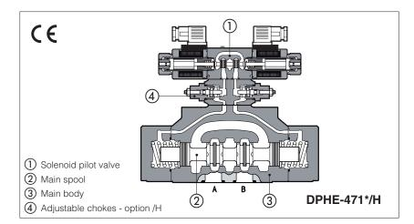
Spool type, pilot operated directional solenoid valves available in 4/3, 4/2, 3/2
