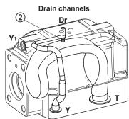
Internal piloting: Without blinded plug SP-X500F ①; External piloting: Add blinded plug SP-X500F ①; Without blinded plug SP-X300F 2; Internal drain: External drain: Add blinded plug SP-X300F 2.
