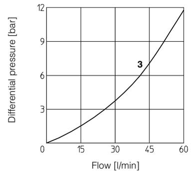
**5 DIAGRAMS OF SKR-0** based on mineral oil ISO VG 46 at 50°C
