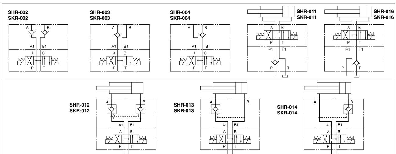
The pilot pressure applied through ports A or B opens the valve acting on ports B and A, respectively. The minimum pilot pressure is a function of the area ratio, see the following table.
